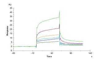
Human TREM2, hFc Tag captured on CM5 Chip via Protein A can bind Biotinylated Human APOE3, His Tag with an affinity constant of 1.41  $\mu$ M as determined in SPR assay (Biacore T200).
